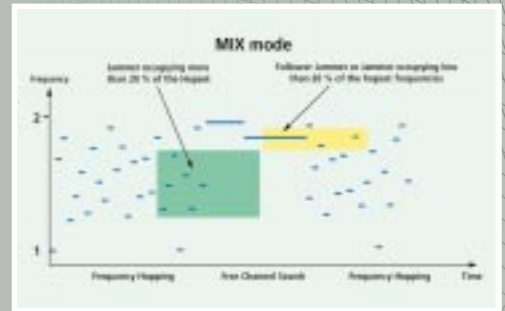
Fig. 1: In mixed FH&FCS mode, radio automatically selects the more appropriate mode, FFH or FCS, according to EW environment.
